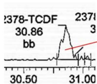
An enlargement of the SICPs of the manually integrated 2378-TCDF ions m/z 303.9016 and m/z 305.8987 from the ICAL standard CS12I as presented in the hardcopy data before manual integration.
